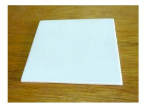
This is the Eze-Kote and glass coated square after spraying with acrylic primer before sanding.
