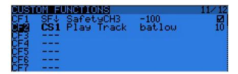
The first column selects the trigger, which can be any switch (physical or custom) or ON (always on). A LONG press of the ENTER key will switch to "toggle" mode (ending with t), i.e. the selected input will be turned on when the selected switch is activated, and will remain on until it is deactivated and reactivated again.
