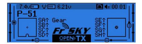
The third shows again the physical switches on the left, and the states of the 32 custom (logic) switches on the right.
