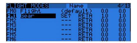
8 flight modes plus the default one are available for use. Each of them can be named, has a selectable activation switch (physical or logical), a trim selection array (R, E, T, A when shown mean the mode has its own trim setting for that control, but each can be changed to a number from 0 to 9 and thus use the same value as the specified mode), and slow up/down parameters for smooth transitions between modes.
