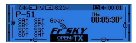
The second shows the gimbal and switches positions, and is handy to check that all the physical controls respond as intended.
