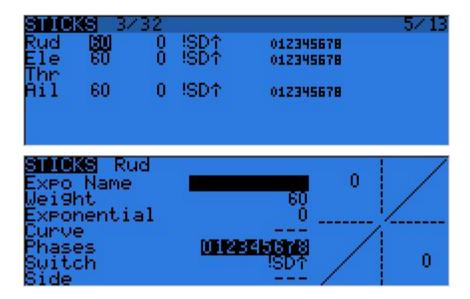
As many lines as required can be assigned to each stick (LONG press ENTER brings up a popup menu to insert/delete lines), and again the first one that has its condition on (starting from the top) will be the active one. This is commonly used to create dual, triple,... rates. A name can be defined for each entry, as well as the rate and exponential ratio. A curve (built-in or custom) can also be used instead of the "simple" exponential function.
