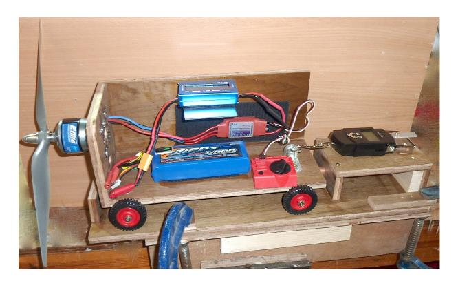
For a range of power settings (300-700W), I recorded: Rpm Voltage (for maximum only) Thrust
