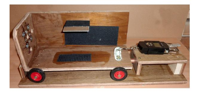
I realised that larger props would need the tester to be raised so I added a base that fits in a bench vice and allows the tester to be g-cramped to it.
