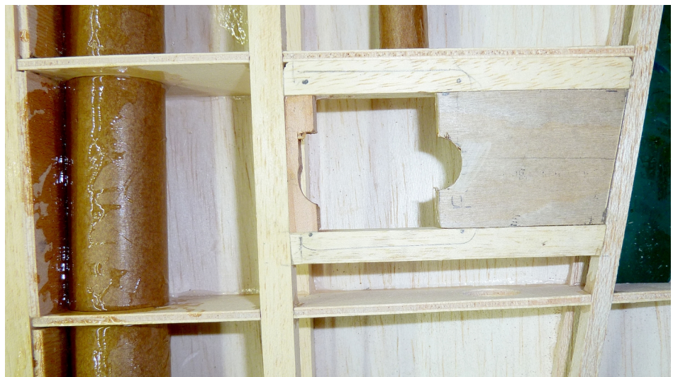
Wing tube fillets and flap servo mount
