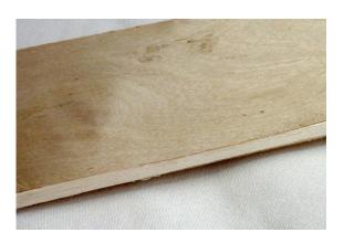
These are the crossed laminations used as a fuselage core in my 2m sloper.
