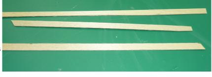
cling film to avoid unwanted adhesion. For the sides I tried thin spruce but, because the parts had both to bend and twist, it wasn't flexible enough. So I cut strips of 0.8mm birch ply. I glued them up in threes with PVA and clamped them in place using pins at each end and clamps in between. I was delighted that the frame turned out very strong and the twisted laminations didn't unbend. Just to be sure I added an intermediate former, before epoxying on the moulding.
