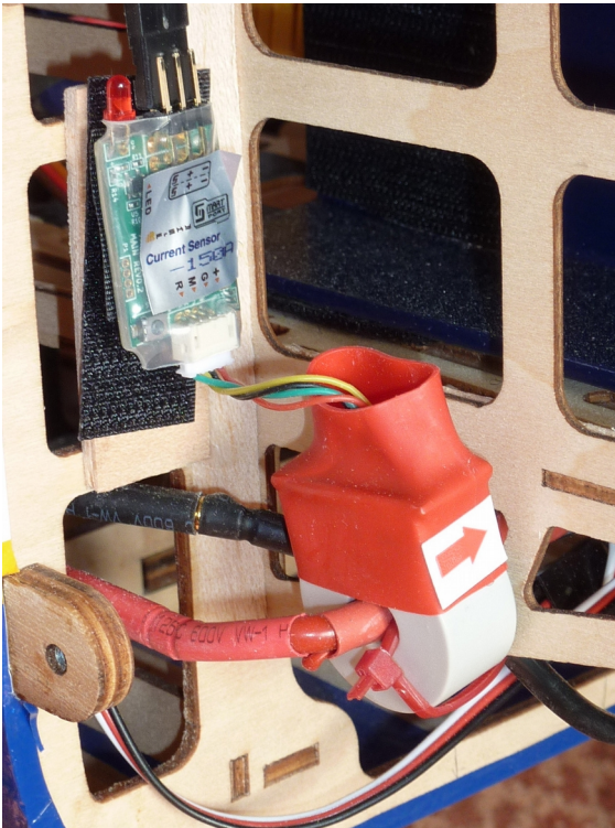
FrSky current sensor and circuit board.
